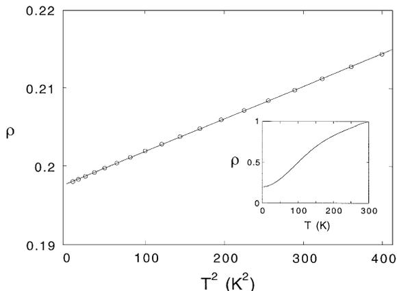
Fig. 1. Plot of  $\rho$  vs  $T^2$  at low temperatures, where  $\rho$  is the resistivity normalized to its value at  $T = 300$  K. Inset:  $\rho$  vs  $T$  up to room temperature.
