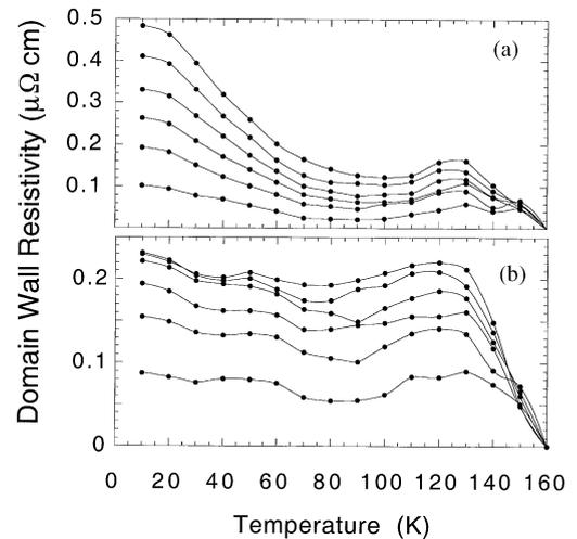
Fig. 1. DWR for different cooling fields from 0 (the top line) to 250 Oe (the bottom line) for currents (a) perpendicular and (b) parallel to the DWs. (The lines are guides for the eye.)
